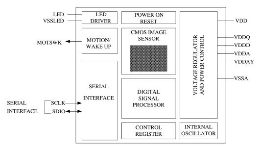
Figure 3. Block Diagram
