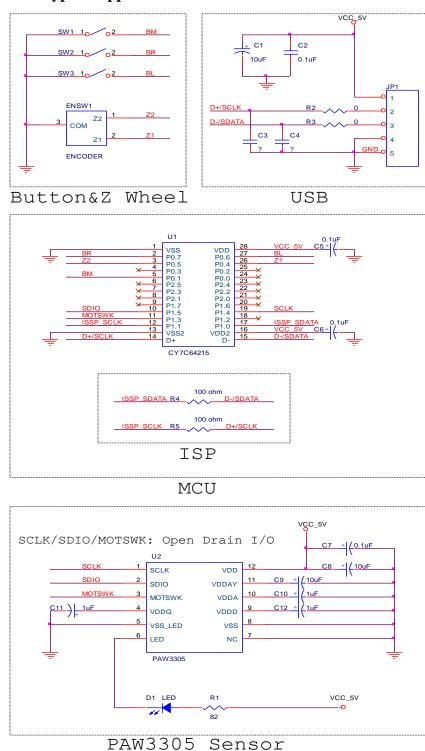
Figure 4. Application Circuit (with Red LED)
